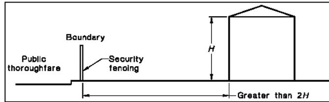
Where the development site adjoins a public thoroughfare, the common boundary between them must be fenced for its full length with a hoarding, unless the least horizontal distance between the common boundary and the nearest parts of the structure is greater than twice the height of the structure. The hoarding must be constructed of solid materials (chain wire or the like is not acceptable) to a height of not less than 1.8m adjacent to the thoroughfare.
