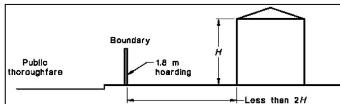
Where a development site adjoins a public thoroughfare with a footpath alongside the common boundary then, in addition to the hoarding required above, the footpath must be covered by an overhead protective structure and the facing facade protected by heavy-duty scaffolding, unless either:
